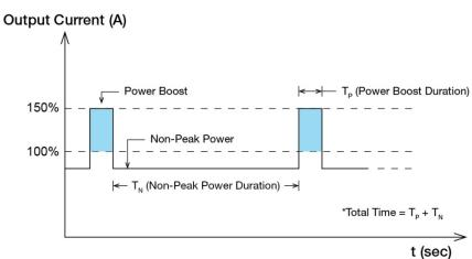
Fig. 3 Duty Cycle Calculation
